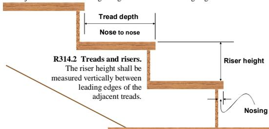
**R314.2 Treads and risers.** The riser height shall be measured vertically between leading edges of the adjacent treads.
