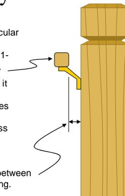
A 2x2 complies with the code requirements for a handrail if it runs continuous the full length of the stairs and the ends are returned.
