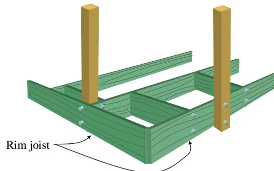
The leverage from a deck railing post will twist the rim joist unless the rim joist is securely fastened to the joist ends or perpendicular blocking. 1/2" lag screws are recommended for resisting code design loads.
